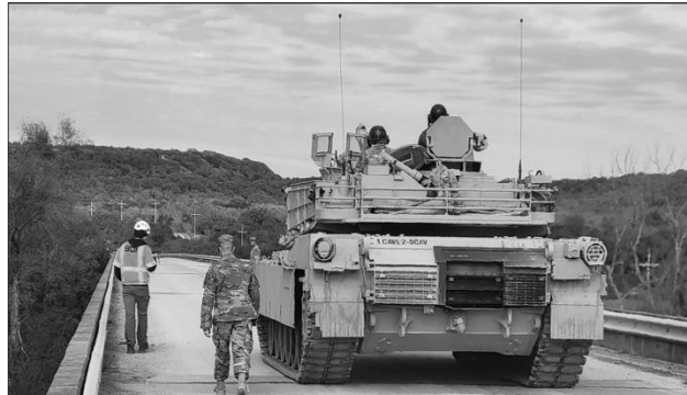
Live Load Testing of Bridges
